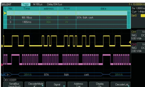
Serial protocol decoding show directly on the waveform with an intuitive, color-coded overlay and presented in binary, hex or ASCII.
