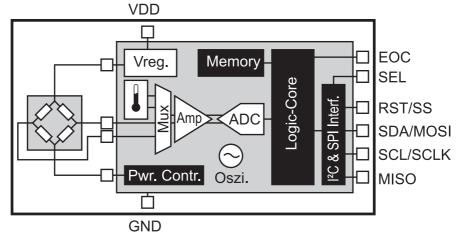
After initialisation the calibration parameters stored in the memory will be transmitted to the MCU (microcontroller unit). Afterwards only the raw pressure and temperature values are transmitted. After a request from the MCU a pressure or/and a temperature measurement is performed. Depending on the accuracy, time and power consumption requirements one out of four different operation modes can be selected before a measurement is executed.
