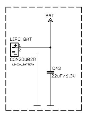
The iMX233 has a built-in battery recharge circuit. This means that if you have a battery and external power supply connected simultaneously, if the battery is not fully charged it would start charging (drawing current from the external power supply).
