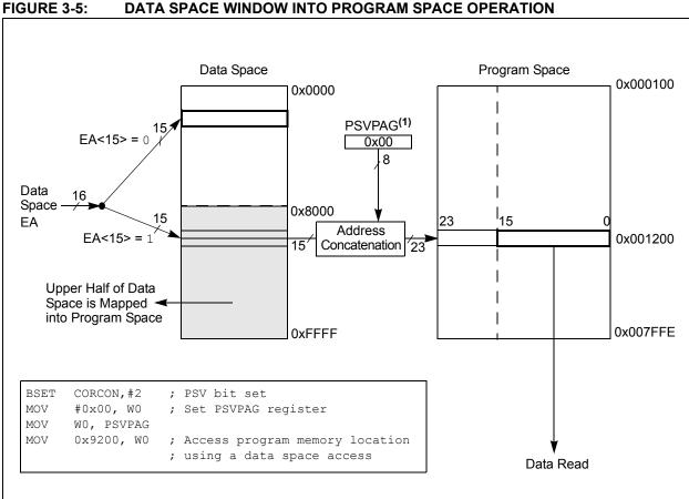
**Note:** PSVPAG is an 8-bit register containing bits <22:15> of the program space address (i.e., it defines the page in program space to which the upper half of data space is being mapped).
