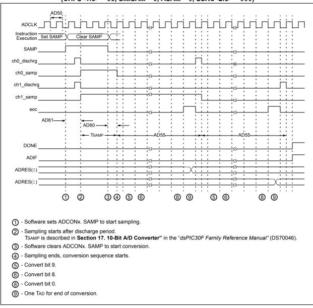
FIGURE 24-25: 10-BIT HIGH-SPEED A/D CONVERSION TIMING CHARACTERISTICS (CHPS<1:0> = 01, SIMSAM = 0, ASAM = 0, SSRC<2:0> = 000)
