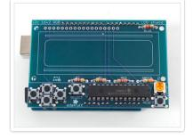
Solder all of the header pins. Even though they aren't used for passing signals, they will make the mechanical connection to the Arduino strong.
