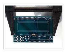
We'll start with the first resistor **R1** - which has yellow, violet, red, gold bands on it. This resistor is part of the interface between the Arduino and the 'port expander' that controls the LCD.
