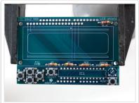
Next up we will place the buttons. These buttons are useful to send a signal to the Arduino (say if you have a basic menu system). We have a 4-way 'direction pad' for up/down/left/right input and a button to the right called SELECT. These 5 buttons should be able to make 'talking' back to your project easy. These are connected to the I2C port expander chip so they require no extra pins on the Arduino, our library does the work of reading whether they are pressed.
