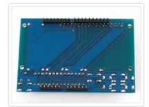
Flip over the shield and place it flat on the table so the long leads of the header stick out.
