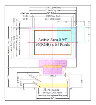
**Note:** The Displays used on our modules are the highest rated 'Grade A' Displays which allow for 0-4 defective pixels.
