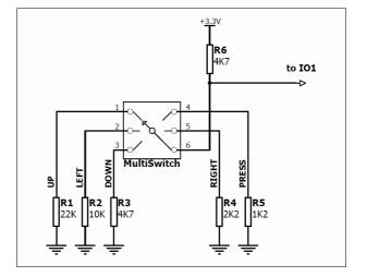
Unused buttons do not need resistors to be connected to the circuit. Table below lists the buttons and corresponding resistor values.
