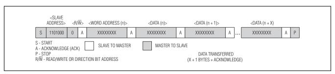
Figure 3. Data Write—Slave Receiver Mode
