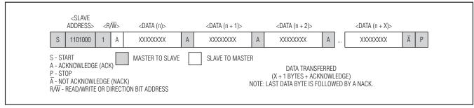
Figure 4. Data Read—Slave Transmitter Mode
