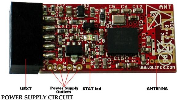
MOD-BT is typically power supplied by UEXT pin 1 and pin 2 with 3.3V.
