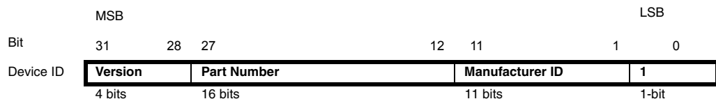
Figure 26-1. The Format of the Device Identification Register
