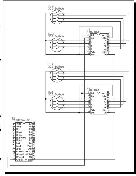
; Sample program to read four BCD switches using 74HCT165 ICs
