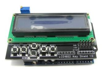
This Arduino 1602 LCD Keypad shield is developed for Arduino compatible boards, to provide a user-friendly interface that allows users to go through the menu, make selections etc. It consists of a LCD1602 white character blue backlight LCD. The keypad consists of 5 keys — select, up, right, down and left. To save the digital IO pins, the keypad interface uses only one ADC channel. The key value is read through a 5 stage voltage divider.
