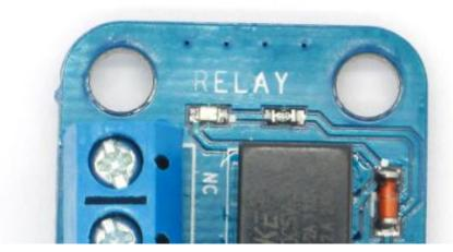
5. Terminals with screws for easy wiring and removing
