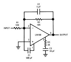
Figure 3. Feedforward Compensation
