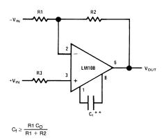
$C_O = 30 \text{ pF}$ \*\*Bandwidth and slew rate are proportional to  $1/C_f$
