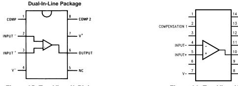
Figure 35. Top View (8-Pin)
