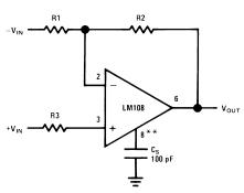
(1) Improves rejection of power supply noise by a factor of ten.
