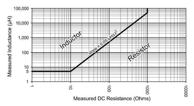
For example, if the inductance of your component is measured at  $100\mu H$  and it has a DC resistance of  $100\Omega$ , then the Atlas LCR will tell you that you have a resistor. If however the resistance was only  $10\Omega$ , then the Atlas LCR will tell you that you have an inductor.
