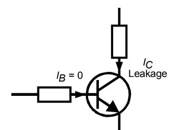
Leakage current Ic=0.17mA Older Germanium types however can suffer from significant collector leakage current, particular at high temperatures (leakage current can be <u>very</u> temperature dependant).
