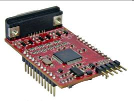
The  $\mu$ VGA-II(SGC) module is a compact and cost effective Serial-to-VGA graphics engine powered by the PICASO-SGC graphics controller. It can provide QVGA/VGA/WVGA graphics solution to any embedded project with its powerful graphics, text, image, animation and countless more features built inside the module.
