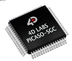
Powerful graphics, text, image, animation and countless more features are built right inside the chip. It offers a simple yet effective serial interface to any host micro-controller that can communicate via a serial port.
