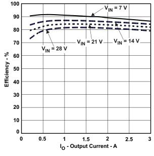
Figure 15. TPS54331 Efficiency
