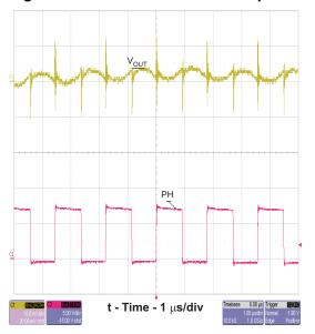
Figure 21. TPS54331 Output Ripple
