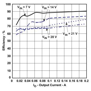
Figure 16. TPS54331 Low Current Efficiency
