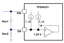
Figure 12. Adjustable Input Undervoltage Lockout
