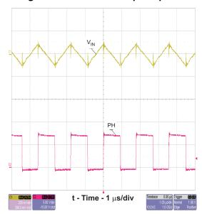
Figure 22. TPS54331 Input Ripple
