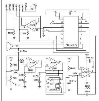
250mS after power-up, the LV-MaxSonar<sup>®</sup>-EZ4<sup>TM</sup> is ready to accept the RX command. If the RX pin is left open or held high, the sensor will first run a calibration cycle (49mS), and then it will take a range reading (49mS). Therefore, the first reading will take ~100mS. Subsequent readings will take 49mS. The LV-MaxSonar<sup>®</sup>-EZ4<sup>TM</sup> checks the RX pin at the end of every cycle. Range data can be acquired once every 49mS.
