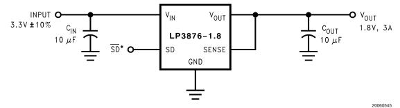
$^\star\overline{SD}$  pins must be pulled high through a  $10k\Omega$  pull-up resistor. See application hints for more information.
