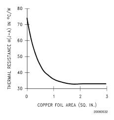
FIGURE 3.  $\theta_{\rm JA}$  vs Copper (1 Ounce) Area for TO-263 package
