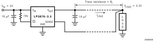
FIGURE 2. Improving remote load regulation using LP3876
