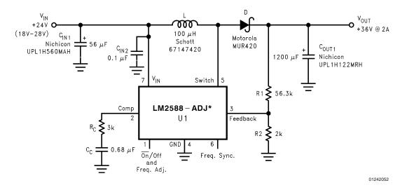
FIGURE 39. +24V to +36V Boost Regulator
