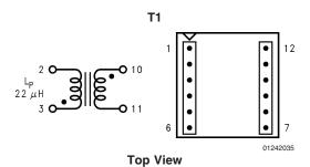
FIGURE 19. Coilcraft Q4435-B (Surface Mount)
