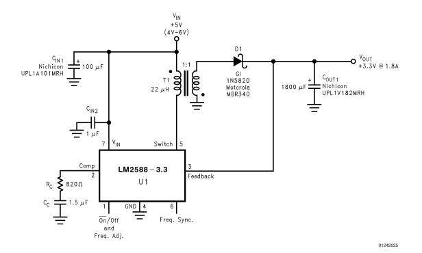
FIGURE 7. Single-Output Flyback Regulator
