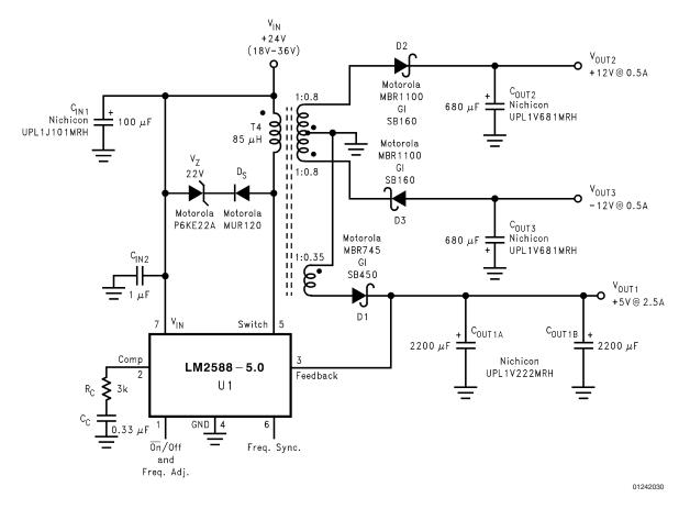
FIGURE 12. Triple-Output Flyback Regulator
