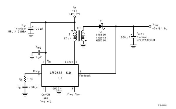
FIGURE 8. Single-Output Flyback Regulator
