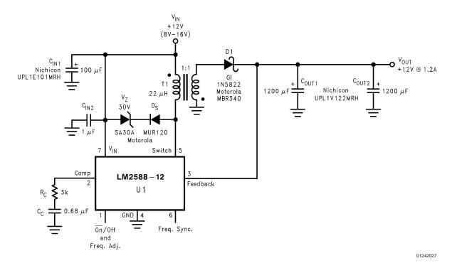
FIGURE 9. Single-Output Flyback Regulator
