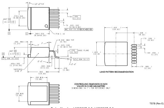
Order Number LM2588S-3.3, LM2588S-5.0, LM2588S-12 or LM2588S-ADJ Tape and Reel Order Number LM2588SX-3.3, LM2588SX-5.0, LM2588SX-12 or LM2588SX-ADJ NS Package Number TS7B
