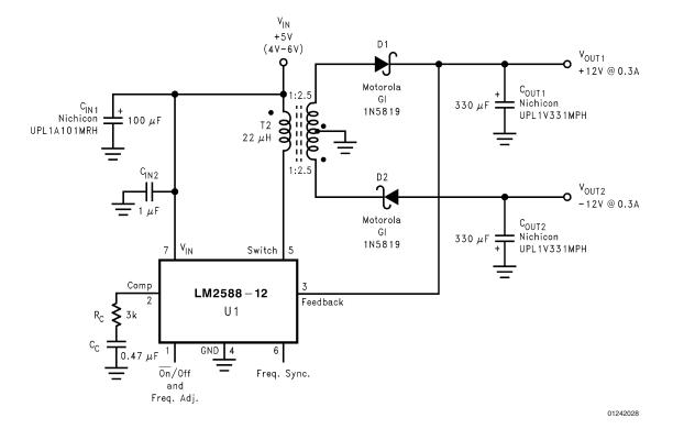
FIGURE 10. Dual-Output Flyback Regulator
