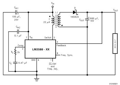
$C_{IN1}-100~\mu F$ , 25V Aluminum Electrolytic $C_{IN2}-0.1~\mu F$  Ceramic $T-22~\mu H$ , 1:1 Schott #67141450D — 1N5820 $C_{OUT}-680~\mu F$ , 16V Aluminum Electrolytic $C_{C}-0.47~\mu F$  Ceramic $R_{C}-2k$
