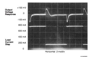
FIGURE 35. V<sub>OUT</sub> Response to Load Current Step
