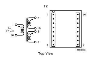
FIGURE 22. Pulse PE-68412 (Surface Mount)
