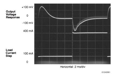
FIGURE 6. V<sub>OUT</sub> Response to Load Current Step
