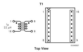
FIGURE 21. Pulse PE-68411 (Surface Mount)
