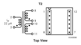
FIGURE 20. Coilcraft Q4436-B (Surface Mount)
