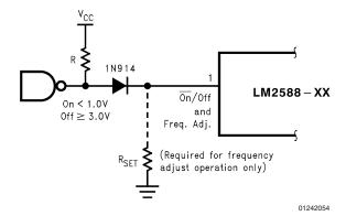
FIGURE 41. Shutdown Operation
