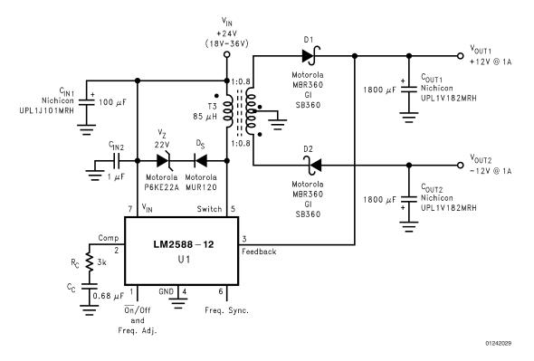
FIGURE 11. Dual-Output Flyback Regulator
