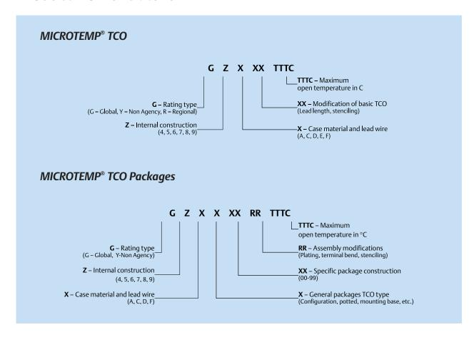
As shown above, Therm-O-Disc MICROTEMP® TCOs follow a consistent product nomenclature that identifies the basic product type, lead wire size, special features and packaging options. For example, a standard G4 series TCO calibrated to open at 192°C would have a part number G4A00192C.
