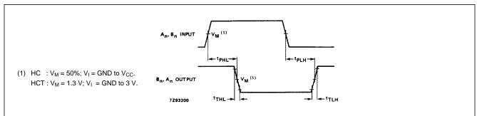
Fig.5 Waveforms showing the input  $(A_n, B_n)$  to output  $(B_n, A_n)$  propagation delays and the output transition times.
