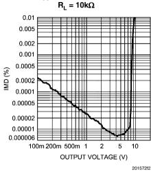
IMD vs Output Voltage  $V_{CC} = 17V$ ,  $V_{EE} = -17V$
