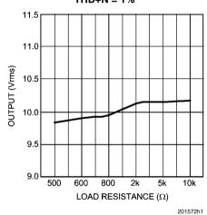
Output Voltage vs Load Resistance  $V_{DD}$  = 17V,  $V_{EE}$  = -17V THD+N = 1%
