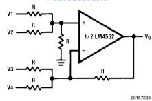
$$V_0 = V1 + V2 - V3 - V4$$
