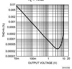
THD+N vs Output Voltage  $V_{CC} = 12V, \, V_{EE} = -12V \\ R_L = 10k\Omega$
