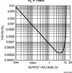
THD+N vs Output Voltage  $V_{CC}$  = 2.5V,  $V_{EE}$  = -2.5V  $R_{I}$  = 10k $\Omega$
