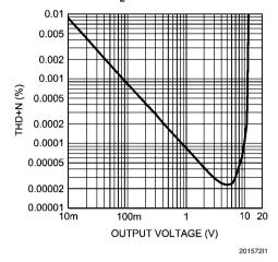
THD+N vs Output Voltage  $\begin{aligned} V_{CC} &= 2.5 \text{V}, \, V_{EE} = -2.5 \text{V} \\ R_L &= 600 \Omega \end{aligned}$
