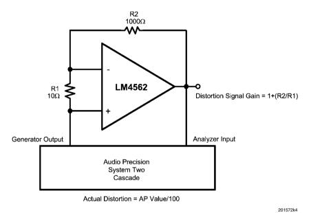
FIGURE 1. THD+N and IMD Distortion Test Circuit
