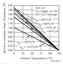
FIGURE 9. Maximum Allowable Power Dissipation vs.
