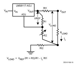
FIGURE 3. Best Load Regulation using Adjustable Output Regulator
