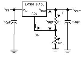
$V_{OUT} = V_{REF} (1 + R2/R1) + I_{ADJ} R2$
