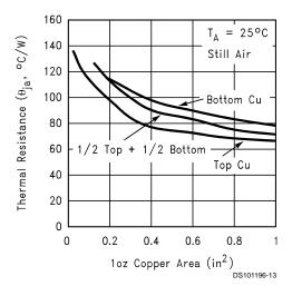
FIGURE 7.  $\theta_{\text{JA}}$  vs. 1oz Copper Area for SOT-223
