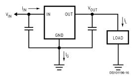
FIGURE 6. Power Dissipation Diagram
