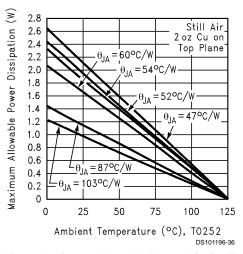
FIGURE 10. Maximum Allowable Power Dissipation vs.
