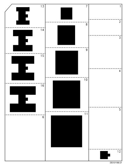
FIGURE 14. Bottom View of the Thermal Test Pattern in Actual Scale
