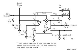
FIGURE 5. Evaluation Board Schematic
