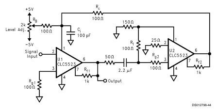
FIGURE 12. Automatic Gain Control Circuit #2
