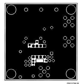
FIGURE 6. DIP Evaluation Board (Top Layer)
