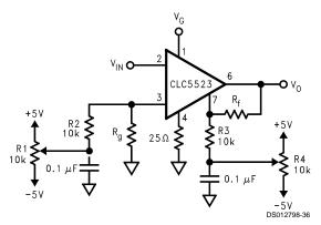
FIGURE 4. Offset Adjust Circuit
