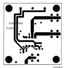
FIGURE 7. DIP Evaluation Board (Bottom Layer)
