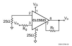
FIGURE 2. Inverting the CLC5523
