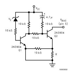
FIGURE 7. External Undervoltage Pull-Down
