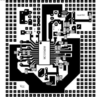
Figure 19. MC13156DW Ground Side Component Placement
