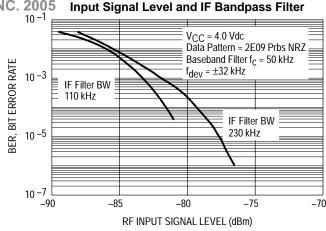
Figure 30. Bit Error Rate versus RF
