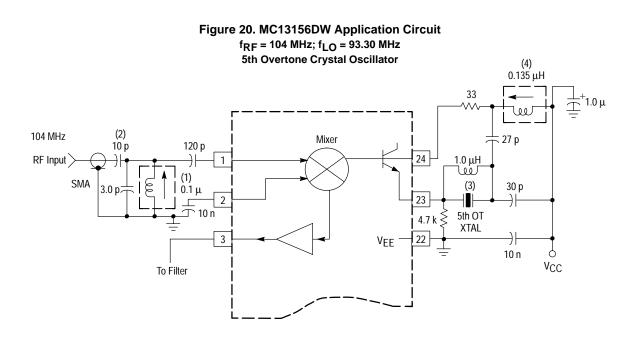
NOTES: 1.0.1 µH Variable Shielded Inductor: Coilcraft part # M1283-A or equivalent. 2. Capacitors are Silver Mica.
