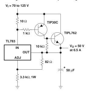
Figure 19. 50-V Regulator With Current Boost
