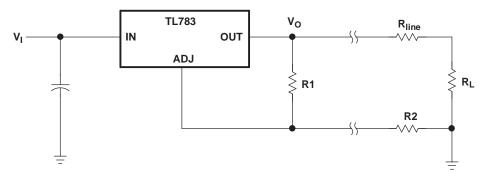
Figure 16. Regulator With Current-Set Resistor
