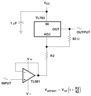
Figure 23. High-Voltage Unity-Gain Offset Amplifier
