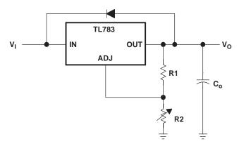
Figure 15. Regulator With Protective Diode
