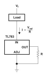
Figure 21. Current-Sinking Regulator
