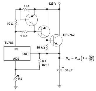
Figure 20. Adjustable Regulator With Current Boost and
