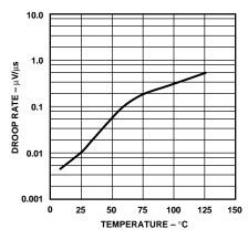
Droop Rate vs. Temperature,  $V_{IN} = 0 V$
