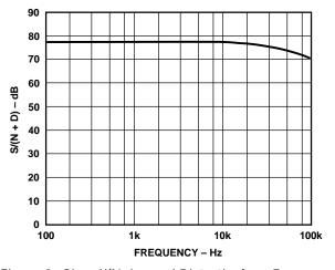
Figure 8. Signal/(Noise and Distortion) vs. Frequency
