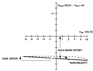
Figure 3. Hold Mode Offset, Gain Error and Nonlinearity
