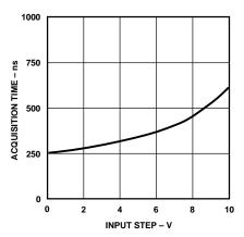
Acquisition Time (to 0.01%) vs. Input Step Size
