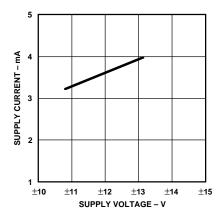
Supply Current vs. Supply Voltage
