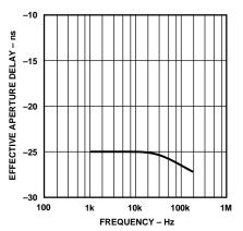
Effective Aperture Delay vs. Frequency
