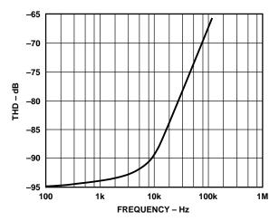
Figure 7. Total Harmonic Distortion vs. Frequency
