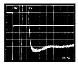
Figure 2. Typical AD781 Hold Mode
