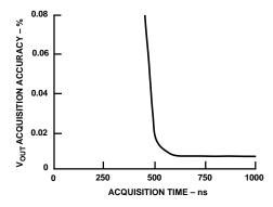
Figure 1. V<sub>OUT</sub> Settling vs. Acquisition Time
