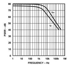
Power Supply Rejection Ratio vs. Frequency
