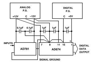
Figure 4. Basic Grounding and Decoupling Diagram
