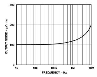
Figure 5. RMS Noise vs. Input Bandwidth of ADC
