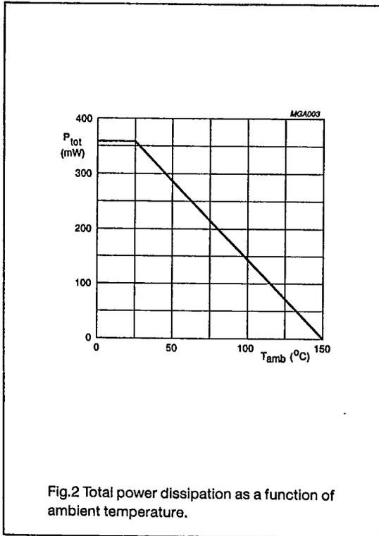
Fig.2 Total power dissipation as a function of ambient temperature.
