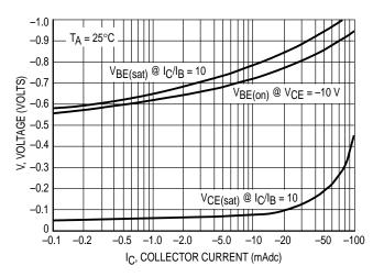
Figure 2. "Saturation" and "On" Voltages
