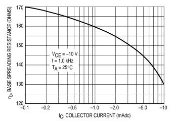
Figure 5. Base Spreading Resistance
