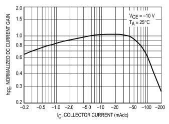
Figure 1. Normalized DC Current Gain
