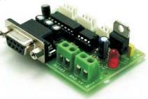
This Kit provides a simple and easy solution to connect your computer to a RS485 Network in either Receiver or Transmitter mode. This kit uses the famous MAX232 and MAX485 interface IC.
