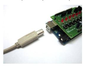
Figure 10. Wiring the USB cable
