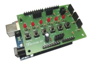
Figure 9. Connecting FK1412 board with Arduino UNO R3 board
