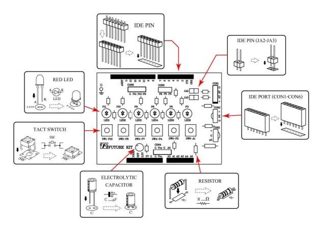
Figure 3. Positioning the parts on PCB
