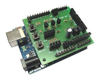
Figure 9. Connecting FK1411 board with Arduino UNO R3 board
