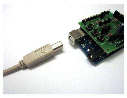
Figure 10. Wiring the USB cable
