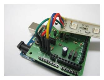
Figure 15. Connecting LED RGB MODULE with FK1411 board
