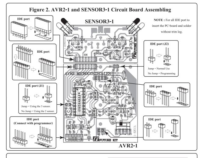
**NOTE:** Jumper J1, If jumping this point is using 2 sensor (left and right side) but if no jumping this point is using 3 sensor (left, right and front side).
