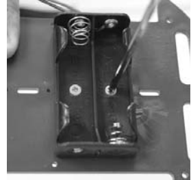
Flat head nut 2.5x10 and NUT M2.5
