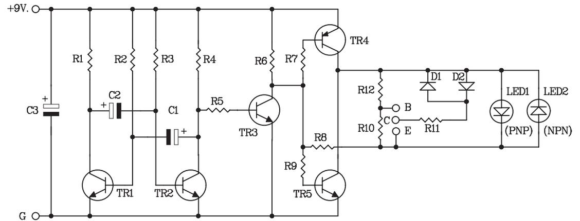
**Figure 2. The in circuit TR checker circuit**
