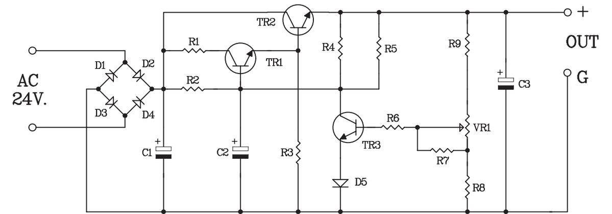
**Figure 2. The variable regulator 0-30V. 1A. circuit**
