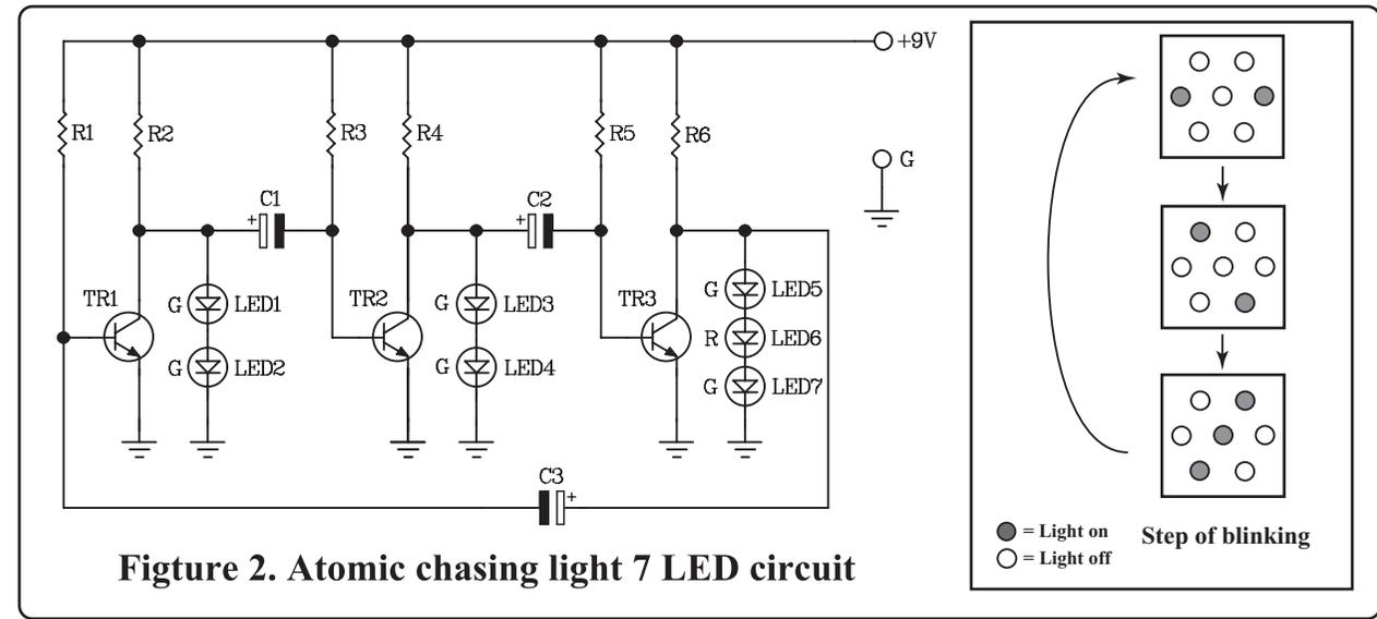
**Figure 2. Atomic chasing light 7 LED circuit**
