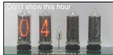
Now you can set the clock. Press and hold the button to advance. After a couple of seconds, the unit advances fast. At release, seconds start from '00'.
