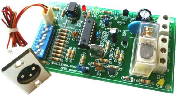
This Kit allows you to control a relay by means of the well-known DMX512 protocol. This protocol was developed by USITT in 1986 to control dimmers, scanners, moving-head spots and other lighting devices with a simple wiring.
