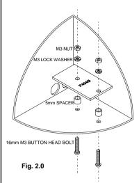
Mount the input PCB on the right-hand side of the housing as shown in the figure. It is possible that a masking sticker from the cabinet will have to be removed, so that one of the supporting bushes can make contact with the cabinet.
