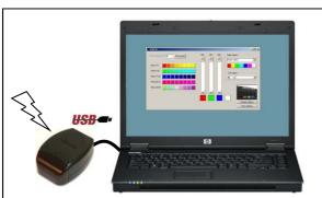
Wireless control from PC also possible with optional K8074 USB to RF converter and free demo software.
