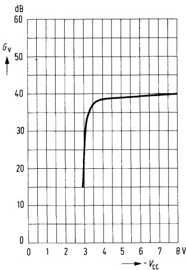
**Voltage gain  $G_V = f(+V_{CC})$**
