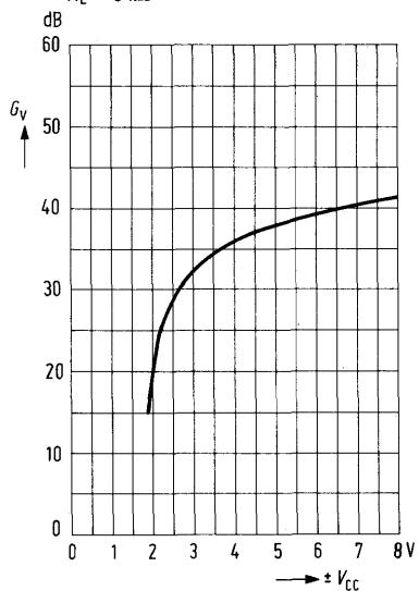
**Voltage gain  $G_V = f(-V_{CC})$**
