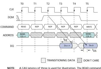
IOTE: A CAS latency of three is used for illustration. The READ command may be to any bank, and the WRITE command may be to any bank.
