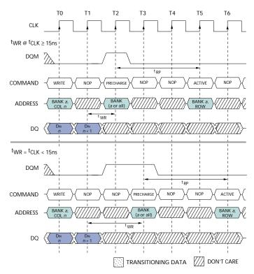
NOTE: DQM could remain LOW in this example if the WRITE burst is a fixed length of two.
