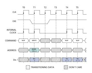
Figure 22 Clock Suspend During WRITE Burst
