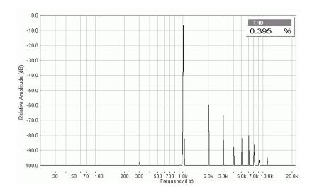
THD @ 750 mW, 12 V supply 8 ohm load G = 20dB
