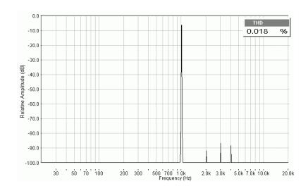
THD @ 100 mW 12 V supply 32 Ohm Load G = 20dB
