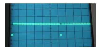
At the Fastest position and using the trimpot P1 to trim for about 99% pulse width. If you over trim then the 556 will 'trip-over' itself and the motor speed will drop. Here is what you see when you just over trim the trimpot from the above photo.
