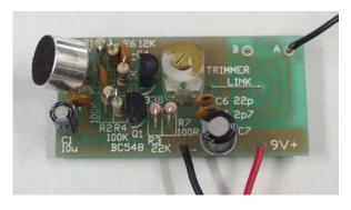
**Power Supply Unit.** The K18 type of transmitter relies upon the effect of variable voltage causing a change of frequency. This means that the PSU must be stable and free from mains hum. A battery is perfect.
